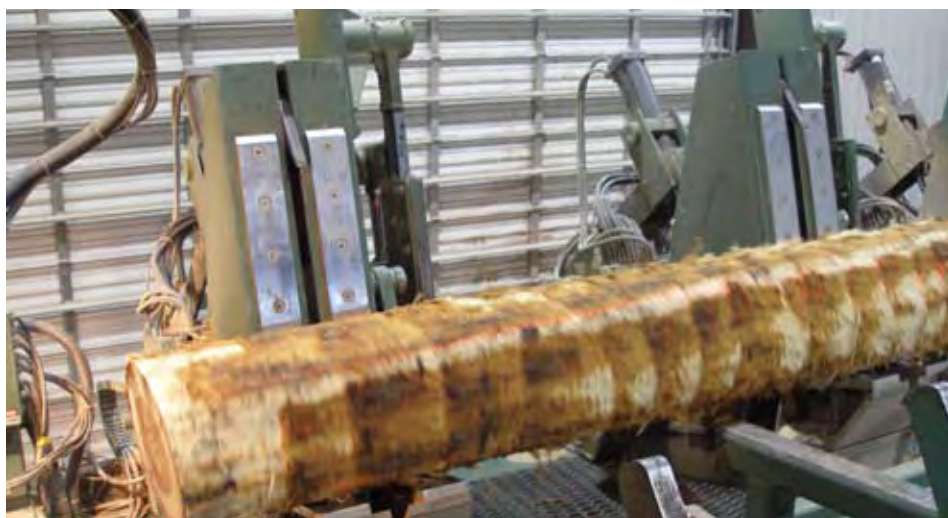
Log is being scanned with USNR’s LASAR hardwood carriage optimizer system.
