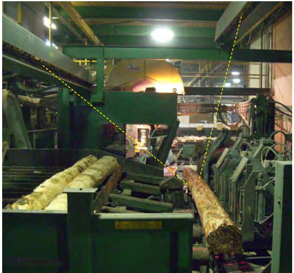
The scanners are positioned above and angled to capture the scan data for the optimized solution.
